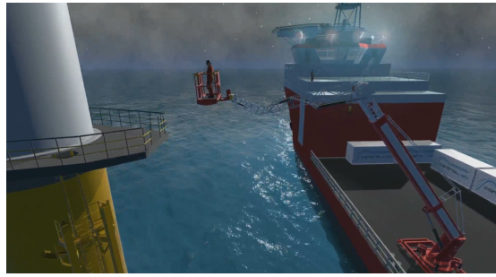
Fig. 3: 3D real-time simulation of a motion compensated crane. Taken from [12].
