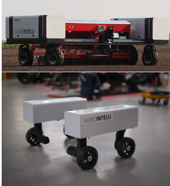
Fig. 19 The Robotti field robot (top) and its small replica (bottom) [45].
